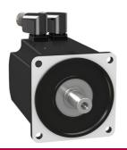
servo motor BMH - 18.5 Nm - 4000 rpm - keyed shaft - without brake - IP54
