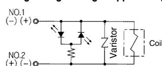
DIN terminal has no polarity.
