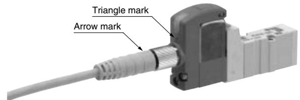
Note) Connector cable should be mounted in the correct direction. Make sure that the arrow symbol on the connector is facing the triangle symbol on the valve when using SMC connector cable (V100-49-1-□). Be careful not to squeeze it in the wrong direction, as problems such as pin damage may occur.
