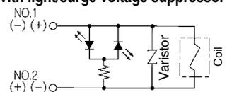
DIN terminal has no polarity.
