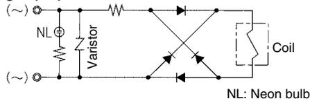
Note) Surge voltage suppressor of varistor has residual voltage corresponding to the protective element and rated voltage; therefore, protect the controller side from the surge. The residual voltage of the diode is approximately 1 V.
