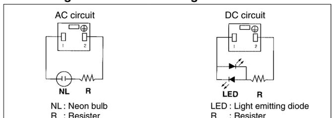
Note) Refer to page 4-4-54 for DIN terminal (Y) conforming to DIN 43650C.
