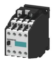
Contactor relay, 44E, DIN EN 50011, 4 NO + 4 NC, screw terminal AC operation 230 V AC 50 Hz, 277 V 60 Hz
