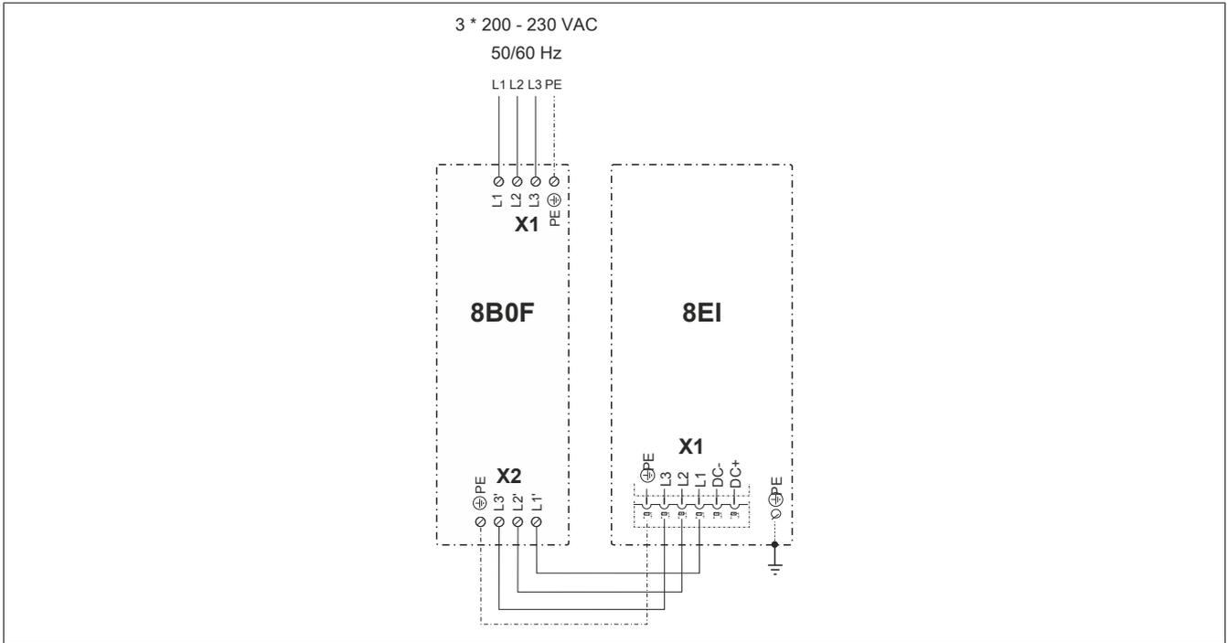
Figure 6: Mains connection 3x 200 - 230 VAC
