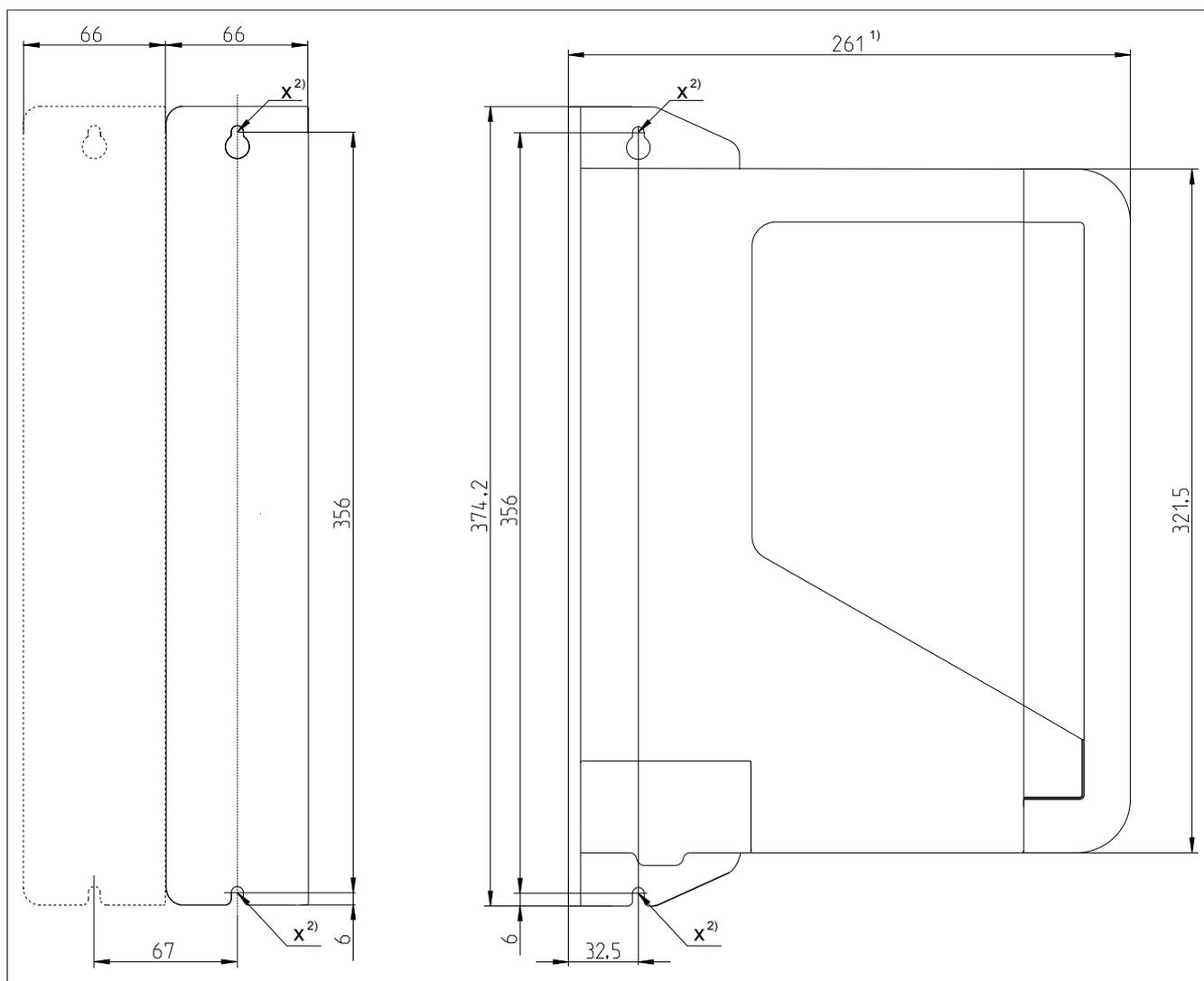
Figure 2: 3-axis modules, single-width - Dimension diagram
