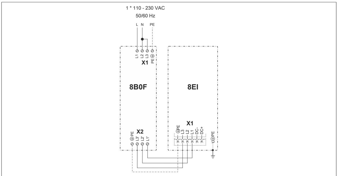
Figure 5: Mains connection 1x 110 - 230 VAC
