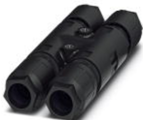
QUICKON H-distributor, black, 4+PE-pos., 2.5 mm 2 ... 6.0 mm 2 /690 V/40 A, for cable diameter of 12 mm ... 20 mm, with a sealing bolt.
