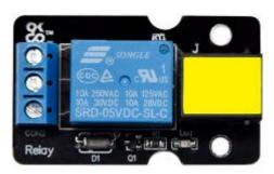
design this relay module with NO (normally open) and NC (normally closed) terminals.
