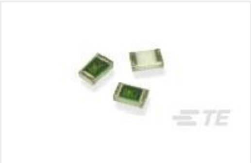
TE Part #7-1614354-5 RN 0603 8K25 0.1% 10PPM CUT LENGTH
