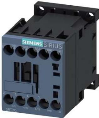
contactor, NEMA version, 5 HP, 460 / 575 V, 3-pole, 24 V AC, 50/60 Hz, auxiliary contacts: 1 NO, screw terminal, size: S00
