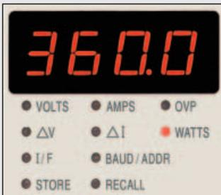
All keyboard entries appear on this display for inspection before they are acted on by pressing the "confirm" key.
