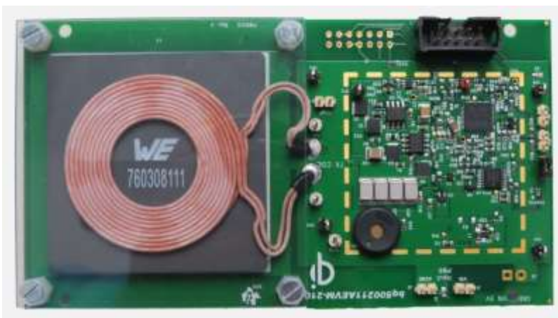
Figure 2: Transmitter board bq500211AEVM-210 from Texas Instruments
