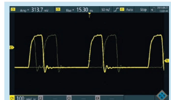
The high-speed acquisition system of the R&S®ScopeRider captures up to 50 000 waveforms/s and uncovers rare and unexpected signal anomalies.
