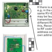
If there is another user nearby, e.g. in the next house, installs the same RV-0356 unit, your receiver may be fault triggered by his/her transmitter. You may select a different RF address code to prevent this. Receiver can only response to RF coding with the same address code setting as its own address code.
