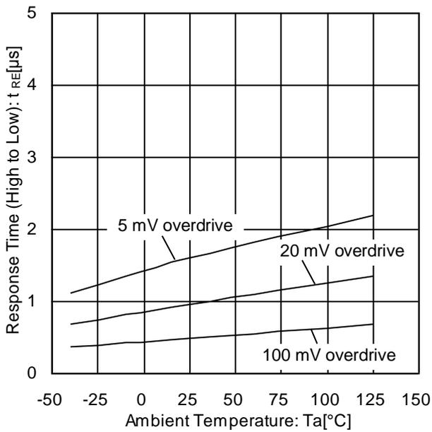
Figure 19. Response Time (High to Low) vs Ambient Temperature
