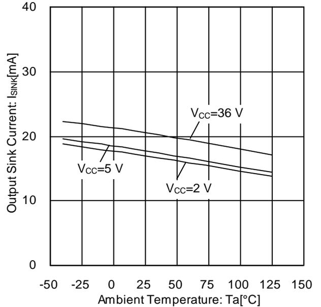
Figure 6. Output Sink Current vs Ambient Temperature (V<sub>OUT</sub>=1.5 V)
