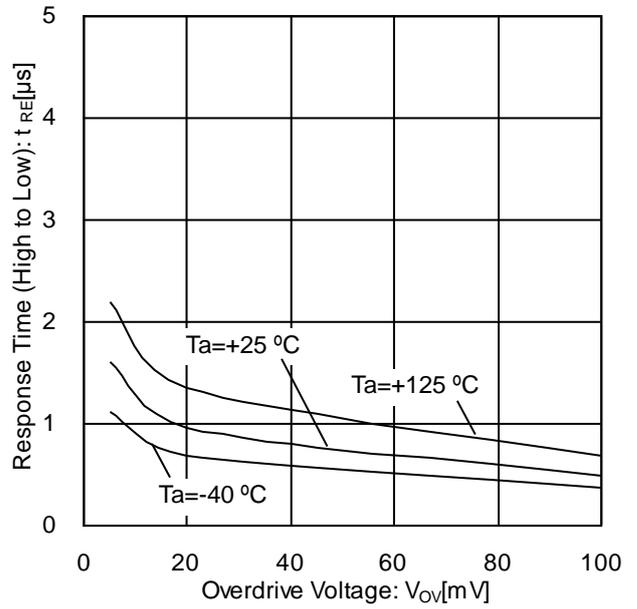
Figure 18. Response Time (High to Low) vs Overdrive Voltage
