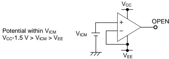
Figure 47. Example of Application Circuit for Unused Circuit
