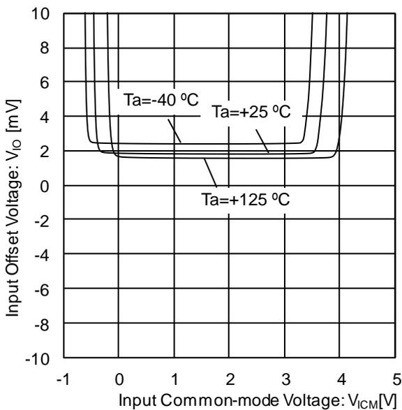
Figure 15. Input Offset Voltage vs Input Voltage (V<sub>CC</sub>=5 V)
