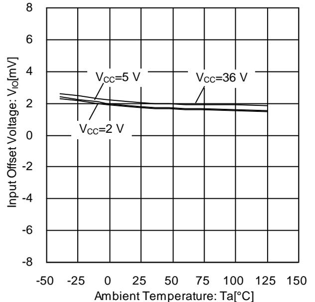
Figure 8. Input Offset Voltage vs Ambient Temperature
