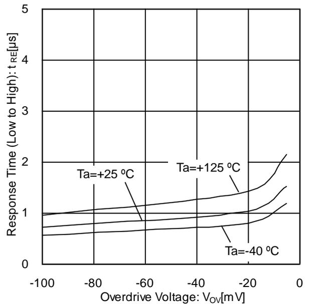
Figure 16. Response Time (Low to High) vs Overdrive Voltage (V<sub>CC</sub>=5 V, V<sub>RL</sub>=5 V, R<sub>L</sub>=5.1 kΩ)
