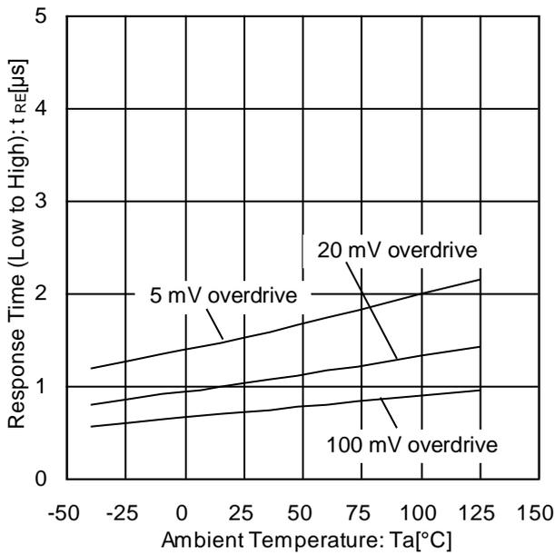
Figure 36. Response Time (Low to High) vs Ambient Temperature
