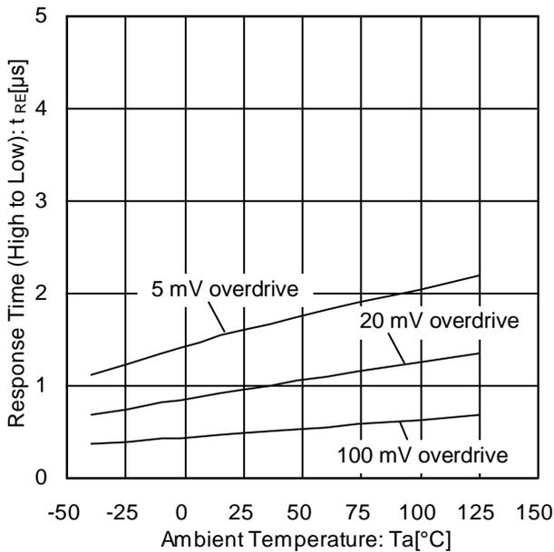
Figure 38. Response Time (High to Low) vs Ambient Temperature
