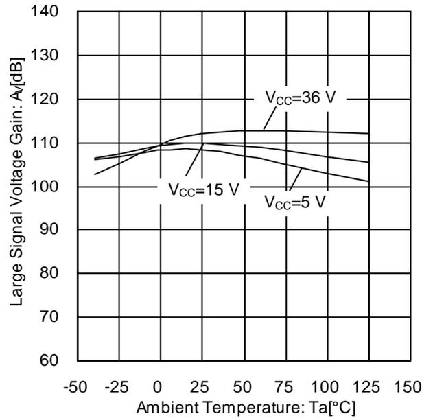
Figure 14. Large Signal Voltage Gain vs Ambient Temperature
