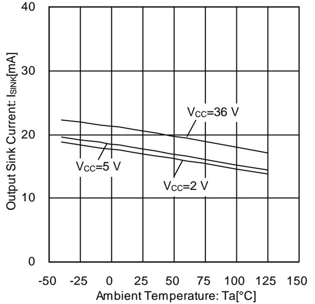
Figure 25. Output Sink Current vs Ambient Temperature (V<sub>OUT</sub>=1.5 V)
