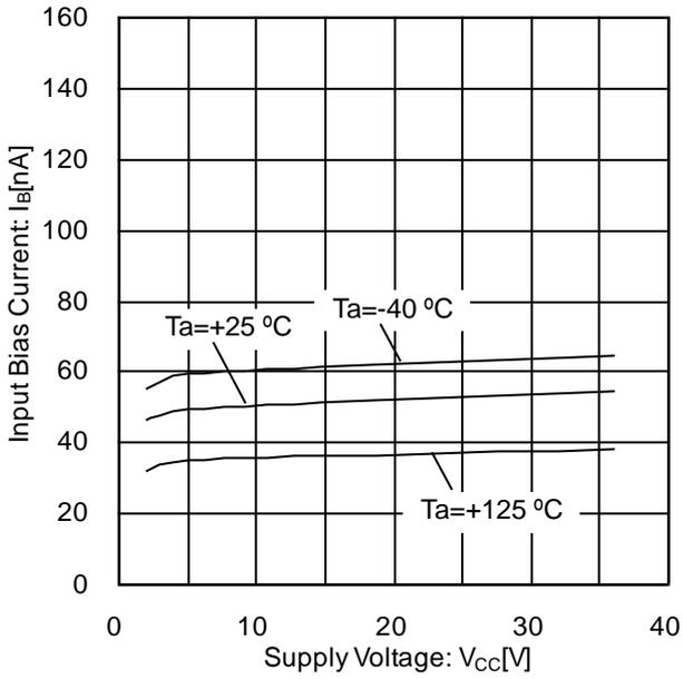
Figure 28. Input Bias Current vs Supply Voltage
