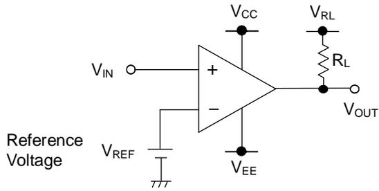
While the input voltage ( $V_{IN}$ ) is higher than the reference voltage, the output voltage remains high. In case the input voltage becomes lower than the reference voltage, the output voltage will turn low.
