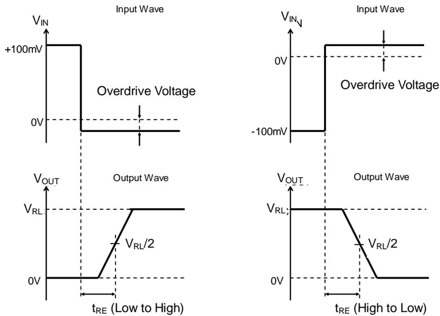
Figure 41. Input / Output Waveform of Response Time
