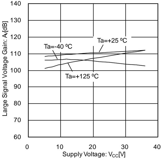
Figure 32. Large Signal Voltage Gain vs Supply Voltage
