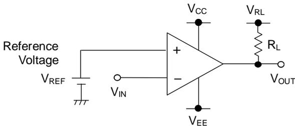
While the input voltage ( $V_{IN}$ ) is lower than the reference voltage, the output voltage remains high. In case the input voltage becomes higher than the reference voltage, the output voltage will turn low.
