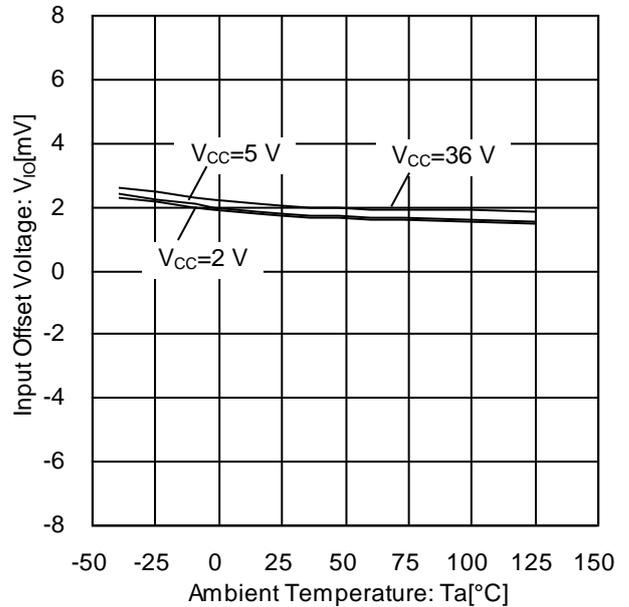
Figure 27. Input Offset Voltage vs Ambient Temperature
