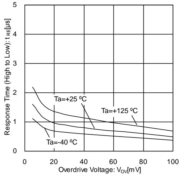
Figure 37. Response Time (High to Low) vs Overdrive Voltage
