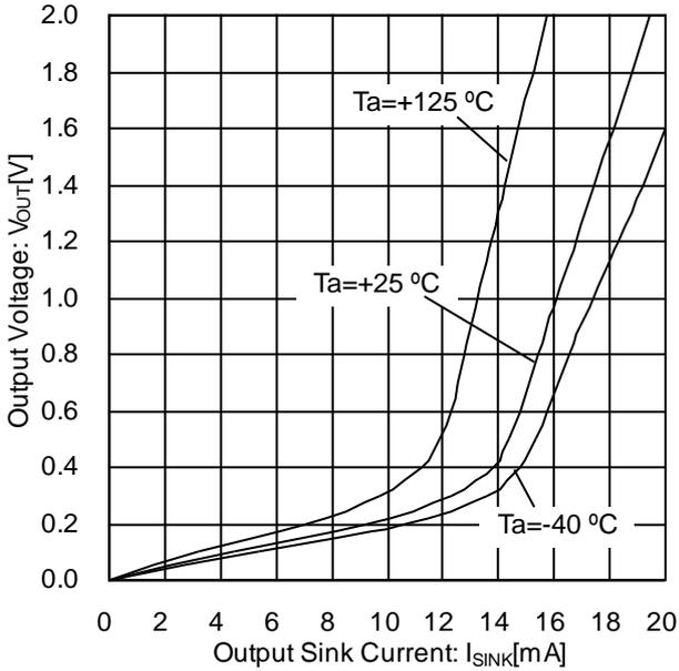
Figure 24. Output Voltage vs Output Sink Current (V<sub>CC</sub>=5 V)
