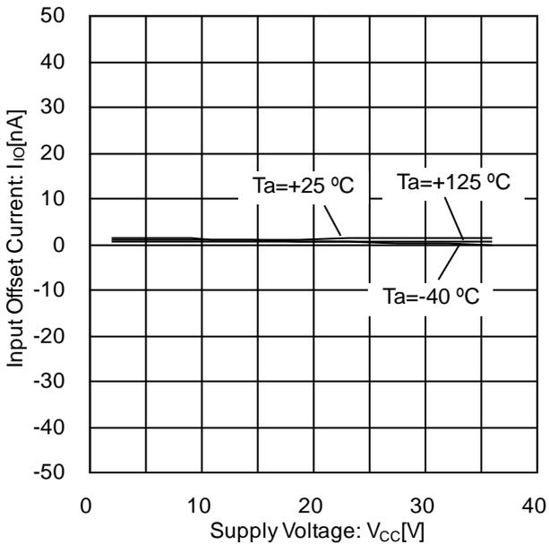
Figure 30. Input Offset Current vs Supply Voltage
