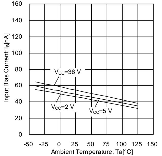
Figure 10. Input Bias Current vs Ambient Temperature
