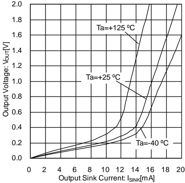
Figure 5. Output Voltage vs Output Sink Current (V<sub>CC</sub>=5 V)
