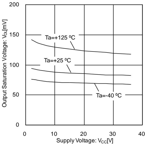
Figure 22. Output Saturation Voltage vs Supply Voltage
