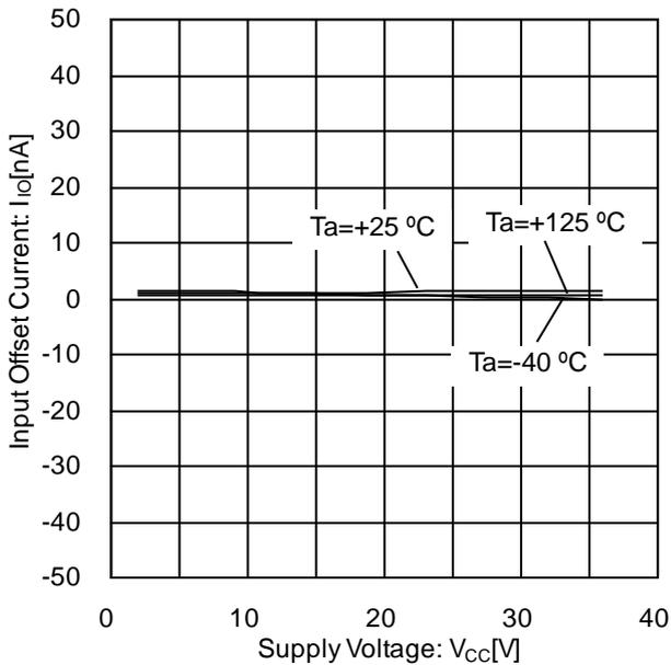
Figure 11. Input Offset Current vs Supply Voltage
