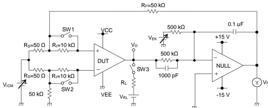
Figure 39. Test Circuit 1 (One Channel Only)
