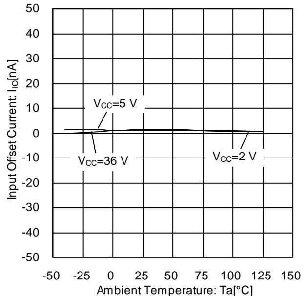
Figure 31. Input Offset Current vs Ambient Temperature
