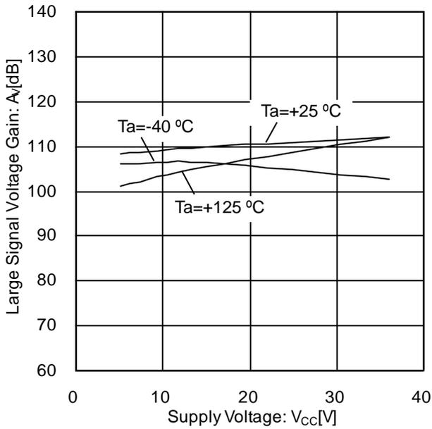
Figure 13. Large Signal Voltage Gain vs Supply Voltage
