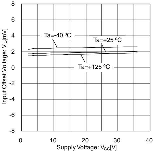
Figure 7. Input Offset Voltage vs Supply Voltage
