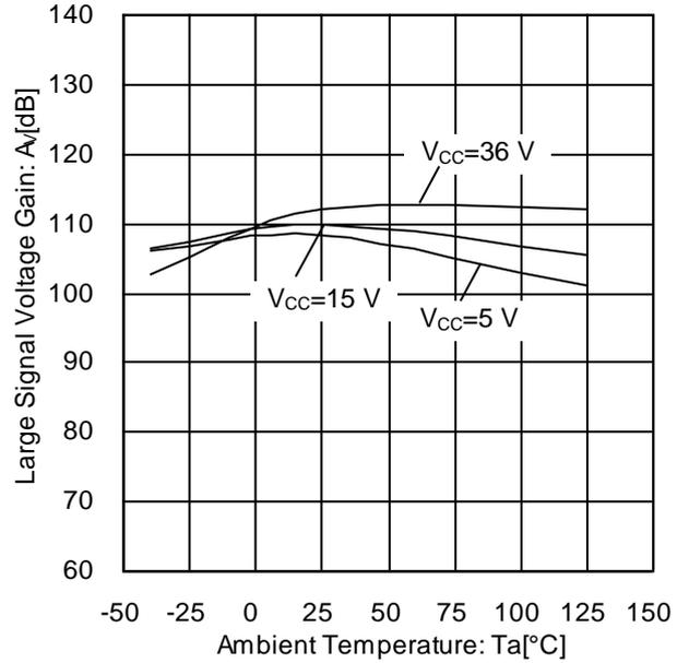
Figure 33. Large Signal Voltage Gain vs Ambient Temperature
