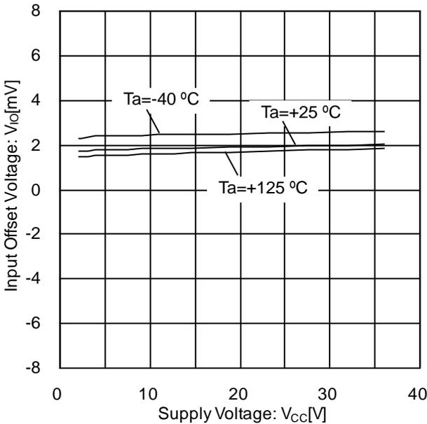
Figure 26. Input Offset Voltage vs Supply Voltage
