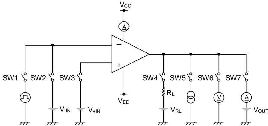
Figure 40. Test Circuit 2 (One Channel Only)
