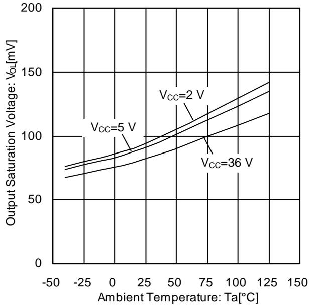
Figure 23. Output Saturation Voltage vs Ambient Temperature
