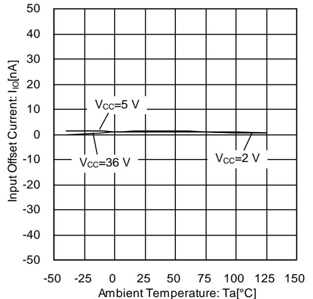
Figure 12. Input Offset Current vs Ambient Temperature
