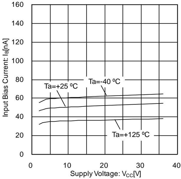
Figure 9. Input Bias Current vs Supply Voltage
