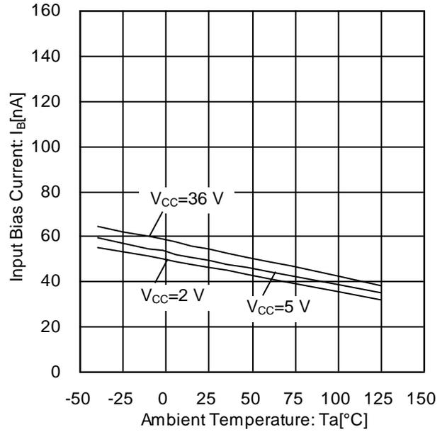
Figure 29. Input Bias Current vs Ambient Temperature
