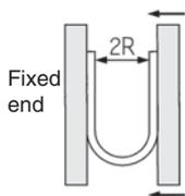
Bend the tube into a U shape at a temperature of 20°C. Fix one end and bend the loop gradually at 100 mm/min. Measure 2R when the tube breaks or is crushed.
