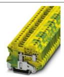
Ground modular terminal block, Connection type: Screw connection, Cross section: 0.14 mm² - 6 mm², AWG: 26 - 10, Length: 57.8 mm, Width: 6.2 mm, Color: green-yellow, Assembly: NS 35/7,5, NS 35/15
