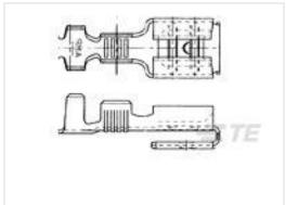
TE Part #160739-4 250 FASTON,PIGGYBACK REC.,18-14 AWG,TPPB
