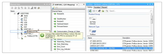
• Right-click on the IF interface and select "Device configuration" to open the configuration environment for the GSD file.
