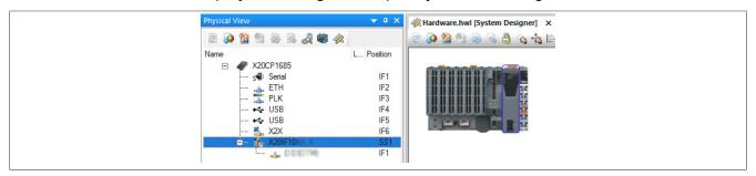
• Additional module settings can be made under "Device configuration". This configuration environment is opened by right-clicking on the IF interface and selecting "Device configuration".
