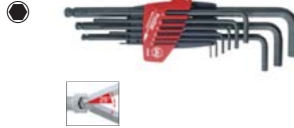
369 S9B Ball end hex L-key set in ProStar. Manganese-phosphated, 9 pcs. Blade: Chrome-vanadium steel, through hardened, manganese-phosphated. Standards: Based on ISO 2936L. Application: Especially for screws that are difficult to access. Extra: Space saving ProStar allows the easy removal of each key without moving any others. The ball end enables the user to work at angles up to 25°.
