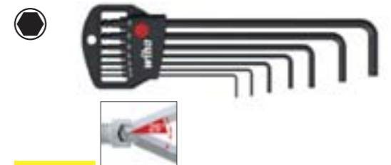
NEW 369 H7B Ball end hex L-key set in holder. Manganese-phosphated, 7 pcs. Blade: Chrome-vanadium steel, through hardened, manganese-phosphated. Standards: Based on ISO 2936L. Application: Especially for screws that are difficult to access. Extra: Popular key sizes kept in a well-organised holder. Simple, rapid operation with solid stopping point for L-keys. The ball end enables the user to work at angles up to 25°.
