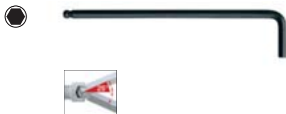
369B Ball end hex L-key, long. Blade: Chrome-vanadium steel, through hardened, manganese-phosphated. Standards: Based on ISO 2936L. Application: Especially for screws that are difficult to access. Extra: The ball end enables the user to work at angles up to 25°.
