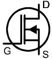
The rare Depletion Mode MOSFET is very similar to the conventional Junction FET (JFET) except that the gate terminal is insulated from the other two terminals. The input resistance of these devices can typically be greater than 1000MΩ for negative and positive gate-source voltages.
