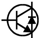
Some transistors, particularly CRT deflection transistors and many large Darlington's have a protection diode inside their package connected between the collector and emitter. The Philips BU505DF is a typical example of a diode
