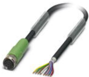
Sensor/Actuator cable, 8-position, PUR halogen-free, Black RAL 9005, shielded, free cable end, on Socket straight M8, Cable length: 5 m
