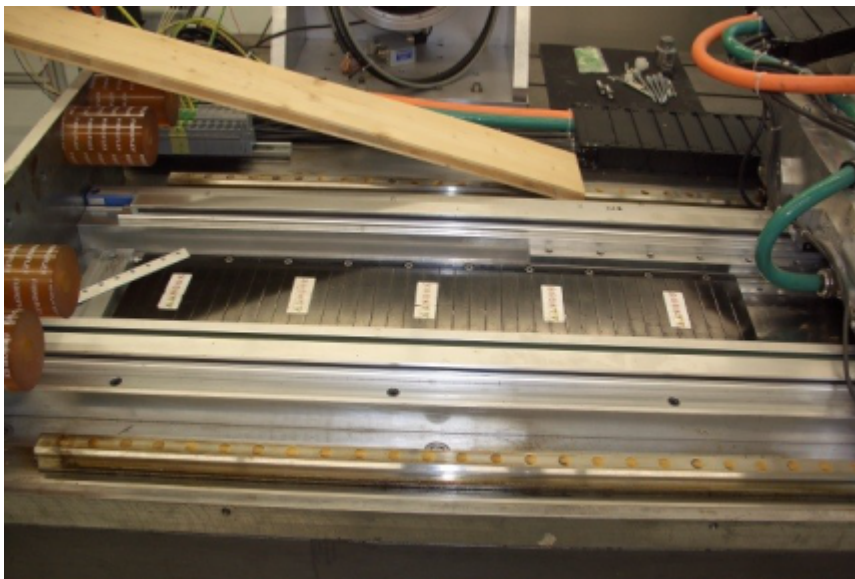
Figure 5-10 Initial situation when mounting the continuous cover band
