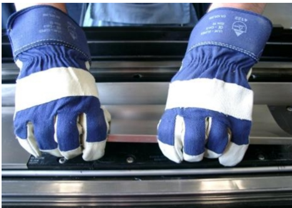
Figure 5-23 Demounting a segment of the segmented secondary section cover
