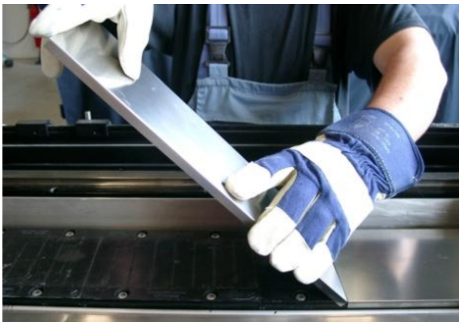
Figure 5-21 Mounting an additional segment of the segmented cover
