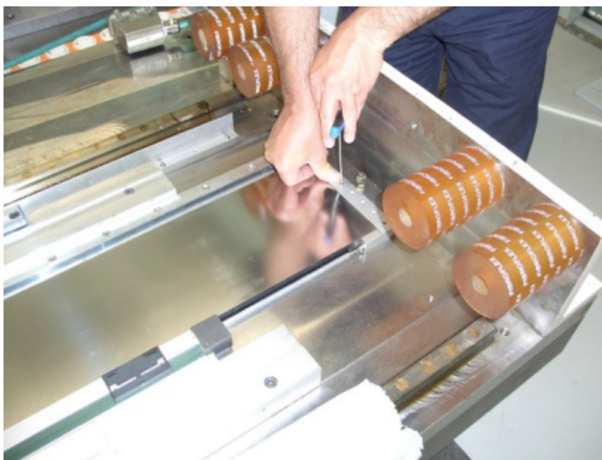
Figure 5-19 Moving up the clamping wedge
