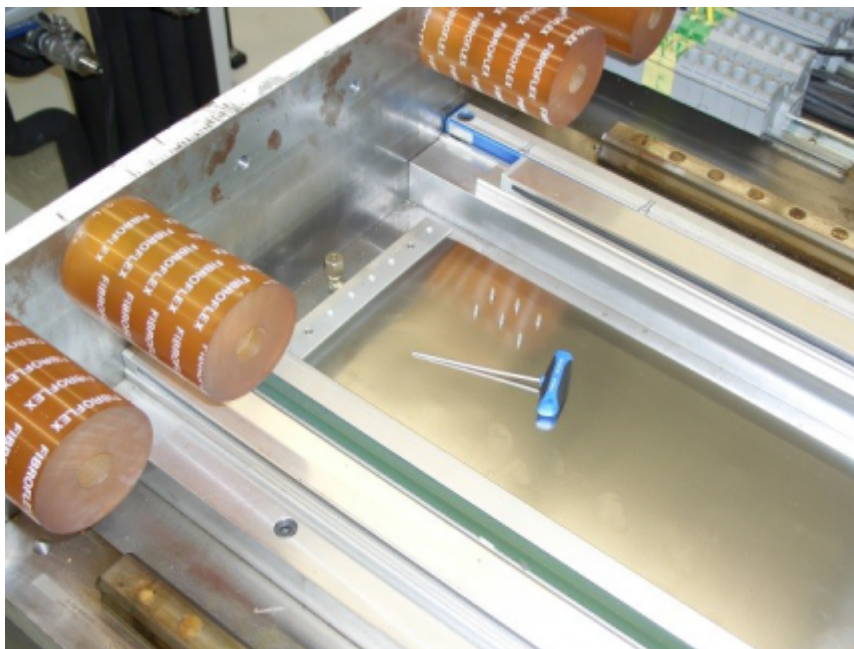
Figure 5-16 Screwing-in the fixing screws
