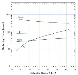
Graph.11 Typical switching losses vs.  $I_c$  T<sub>j</sub>=175°C,  $V_{cc}$ =600V, L=500 $\mu$ H  $V_{ce}$ =15V,  $R_e$ =10 $\Omega$
