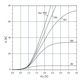
Graph.5 Typical Transfer Characteristics  $V_{ce}$ =+15V
