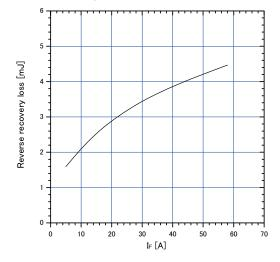
Graph.14 Typical reverse recovery characteristics vs.  $I_F$   $T_j$ =175°C,  $V_{\infty}$ =600V, L=500 $\mu$ H,
