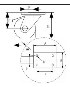
Castor Assembly: Pressed stainless steel -AISI 304-. Swivel on two rows of balls.
