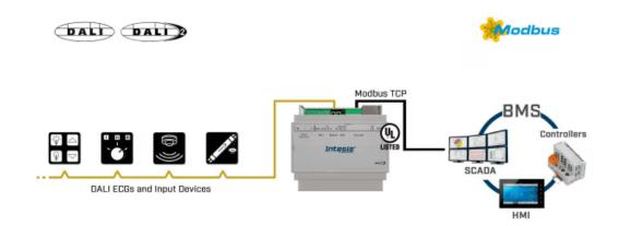
Integration of DALI drivers and sensors into a Modbus installation.
