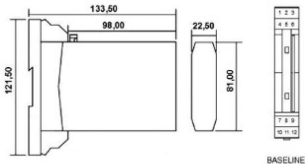
Dimensions: width: 22,5 mm - Height: 81 mm - Depth: 98 mm
