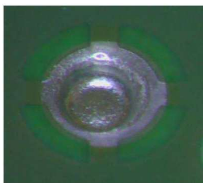
Soldered Shield Pin 焊接屏蔽引脚
