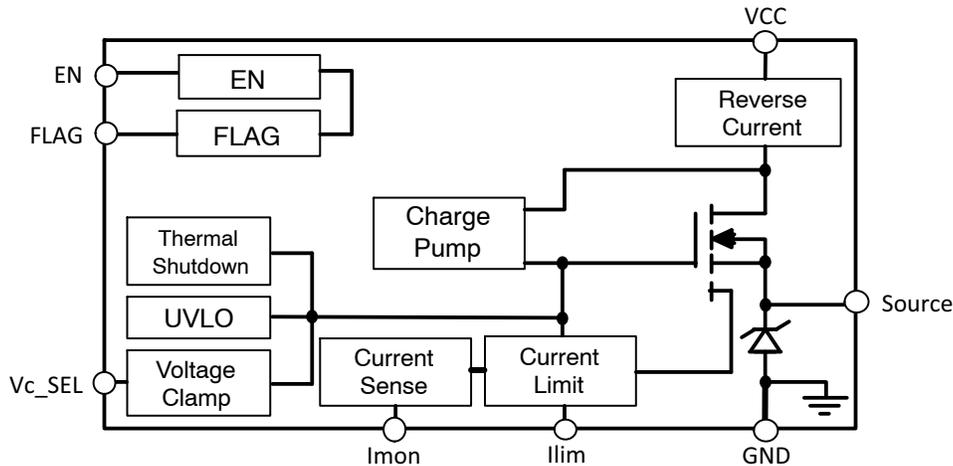
Figure 2. Block Diagram
