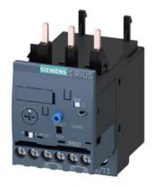
Overload relay 1...4 A Electronic For motor protection Size S0, Class 20 Contactor mounting Main circuit: Screw Auxiliary circuit: Screw Manual-Automatic-Reset
