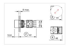
A = Plug-in terminal 2.8 mm x 0.5 mm C = Screw terminal E = Slow-make switching element F = Snap-action switching element
