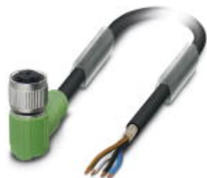
Sensor/Actuator cable, 4-position, PUR halogen-free, black-gray RAL 7021, shielded, free cable end, on Socket angled M12 SPEEDCON, A-coded, Cable length: 10 m
