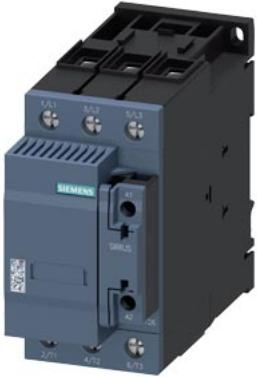
capacitor contactor, AC-6b 75 kVAr, / 400 V, 3-pole, 110 V AC, 50 Hz, auxiliary contacts: 2 NC, screw terminal, size: S2
