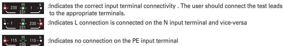
If the wiring condition is other than normal, the Tester is limited on its measurements that can be performed.
