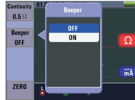
**F1 Button:** Pop-up and shutdown LOW OHM menu, Shutdown mode is activated when the user selects.
