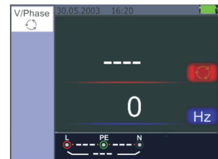
Figure 21 Initial screen of the Phase Sequence Measurement
