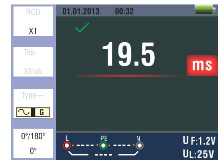
Figure 17x1 Mode-Measuring screen
