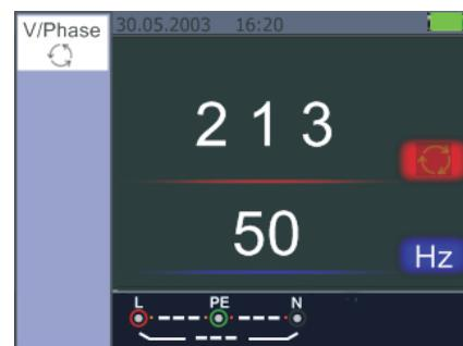
Figure 24 Phase Sequence-When connected in counter-clockwise manner
