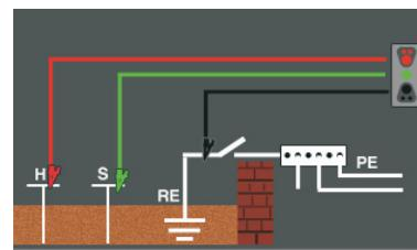
**6.4-Earth Resistance Display/Switch and Terminal Settings**
