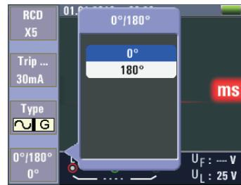
**F1 Button:** Pop-up and shutdown RCD menu, Shutdown mode is activated when the user selects.
