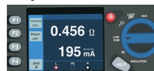
A continuity test is used to verify the integrity of connections by making a high resolution resistance measurement. This is especially important for checking Protective Earth connections.
