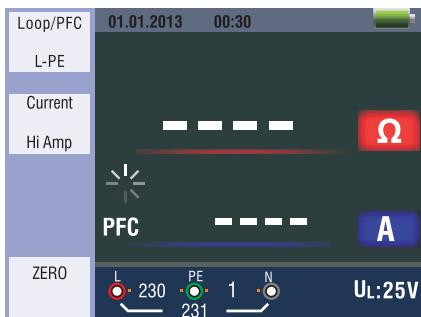
Figure 7 Hi Amp LOOP-To be used where NO RCD is present
