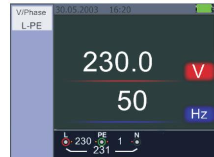
Figure 20 Screen while measuring Voltage and Frequency
