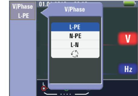
**F1 Button:** Pop-up and shutdown Voltage/Phase menu, Shutdown mode is activated when the user selects.
