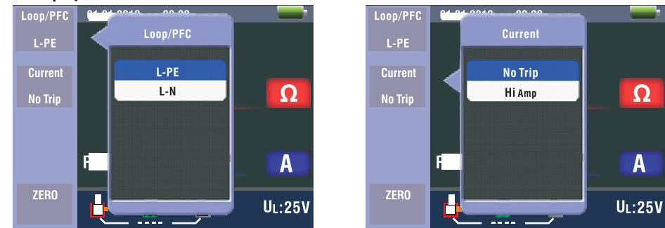
**F1 Button:** Pop-up and shutdown Loop/PFC menu, Shutdown mode is activated when the user selects.
