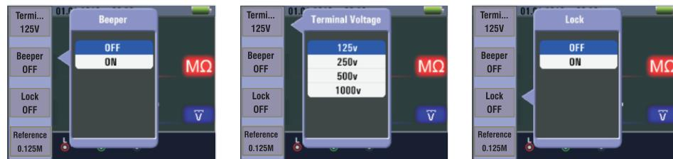
**F1 Button:** Pop-up and shutdown Insulation menu, Shutdown mode is activated when the user selects.
