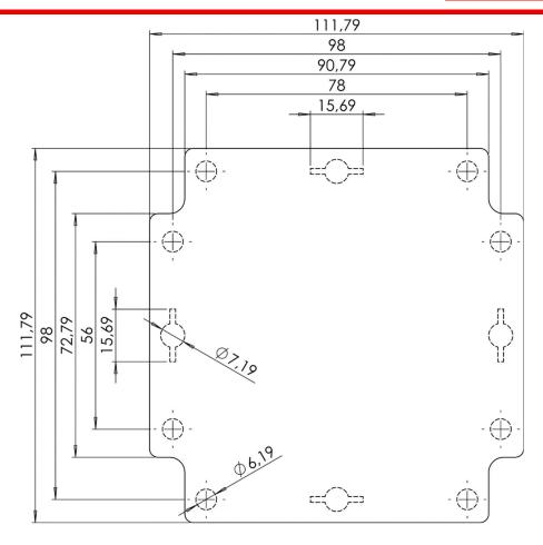
Dashed line shows outline of the mounting boss under PCB board Recommended mounting holes diameter ø2,6mm All dimensions are given within +/-0,5mm tolerance
