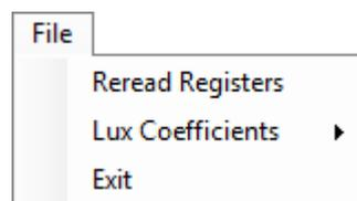
The **Reread Registers** function forces the program to re-read all of the control registers from the device and display them on the screen. This does not read the output data, because the program reads those registers continually while it is running.
