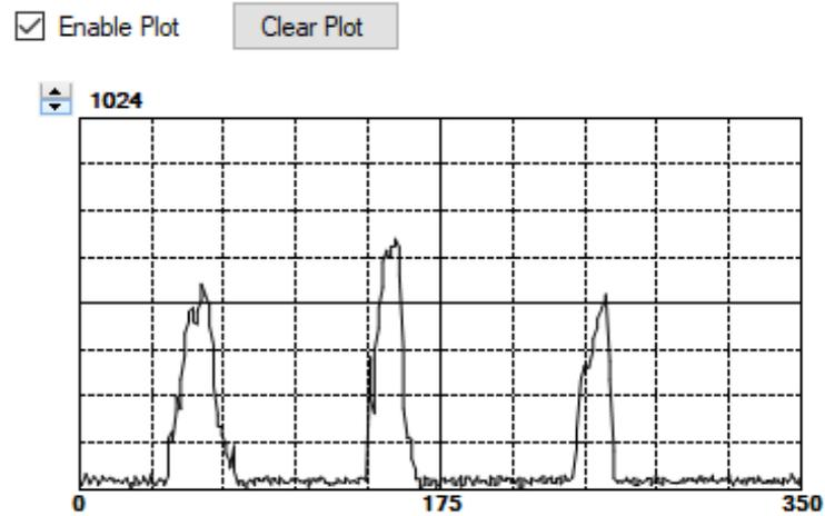
The scale of the Y-axis of the plot can be adjusted by clicking on the small up and down arrows at the top left corner of the plot. The scale can be set to any power of 2 from 16 to 16384.
