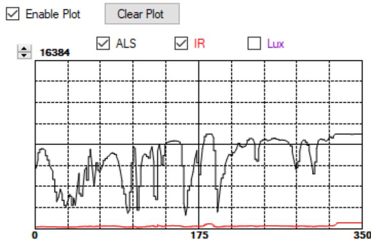
The scale of the Y-axis of the plot can be adjusted by clicking on the small up and down arrows at the top left corner of the plot. The scale can be set to any power of 2 from 64 through 65536.
