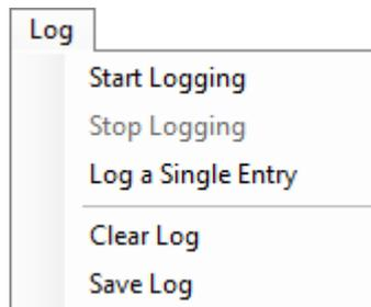
Click **Start Logging** to start the logging function. Each time the program polls the output information from the device, it creates a new log entry showing the raw data values, the values of various control registers, and the values entered by the user into the text fields near the bottom right corner of the window.
