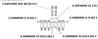
The AKZ 4 terminal include the option of setting up a cross-connection with more than 10 poles, e.g. 20-pole:
