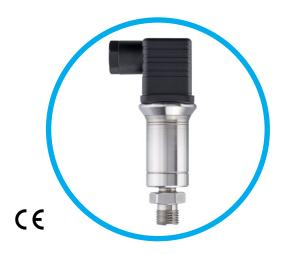
The external mount hydrostatic level transmitter, ILSE, has a piezoresistive silicon pressure sensor which is an oil filled isolated diaphragm. The sensor and housing are made from stainless steel with a choice of internal O ring seals to ensure the product is suitable for a wide range of applications.
