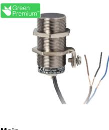
Inductive proximity sensors XS ATEX D, inductive sensor hazardous area, M30, Sn15mm, 12...48 VDC, NC, cable 10 m
