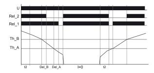
Example: I=0 Inv. with minimum monitoring (2MIN+I=0 ON)
