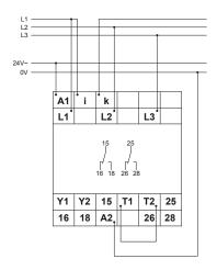
Connected 3~ 400V with power module 400V AC with fault latch I<sub>N</sub><12A
