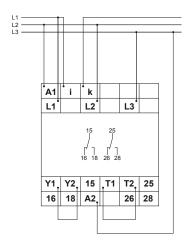
Connected 3~ 400V with power module 400V AC with fault latch and temperature monitoring sensor  $I_{\text{N}} {<} 12A$
