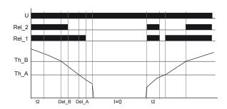
Example: I=0 with maximum monitoring (2MAX+I=0 ON) relay state normal: Rel\_1 and Rel\_2 off
