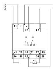
Connected 1~ 230V with power module 230V AC without fault latch but with current transformer  ${\bf I_h}{>}{\bf 12A}$
