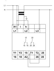
Connected 3~ 400V with power module 400V AC with fault latch and current transformer  $I_{N}\!\!>\!\!12A$
