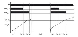
Example: I=0 Inv. with maximum monitoring (2MAX+I=0 ON) relay state invers: Rel\_1 and Rel\_2 on
