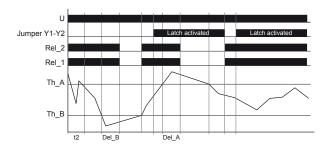
Example: Window function (WIN) - Resetting the fault latch by pressing the plus- and minus-key (+ & -)
