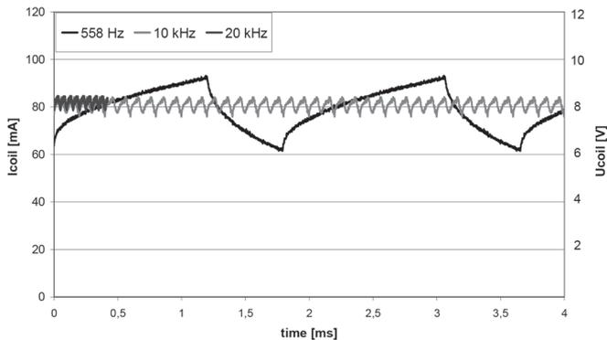
Figure 3: Effect of different PWM frequencies on ripple coil current on Power F relay with parallel diode
