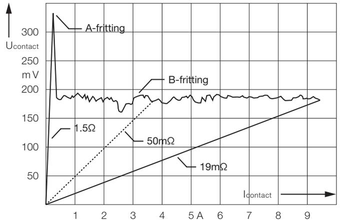
Fig. 2 Fritting of a relay contact
