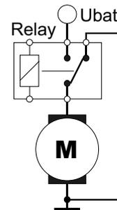
Fig. 1 Short-circuit brake
