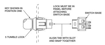
NOTE: Switch installation is permanent. Switch cannot be removed from lock after assembly. Attempts to separate switch and lock may damage switch.
