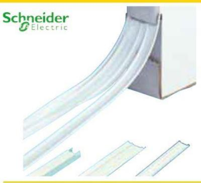
Boxed/Coiled mini trunking has been designed for ease of transport. 15Mtr coils in either non adhesive or self adhesive style. Simply pull from the box, the trunking sides fold upwards and take the shape of the trunking. Accessories below/next page.
