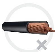
Pulled out conductor
