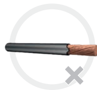
Insulation not cut in properly
