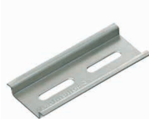
TS 15/5.5 mm according to EN 60715 (s = 1.0 mm)
