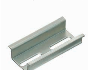
TS 35/15 mm according to EN 60715 (s = 1.5 mm)
