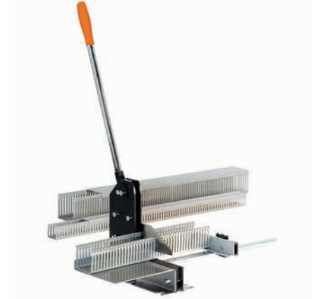
Wire channel cutter for manual operation in cutting wiring channels and covers up to 125 mm wide and a wall thickness of 2.5 mm. Not suitable for plastics reinforced by fillers plastics.
