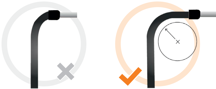
Risk of breakage due to overload
