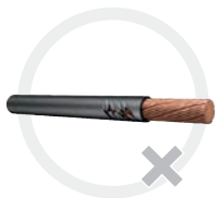
Damaged conductor insulation
