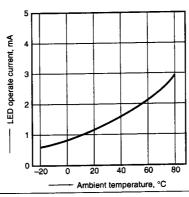
6. LED turn off current vs. ambient temperature characteristics Sample: All types; Load voltage: Max. (DC); Continuous load current: Max. (DC)
