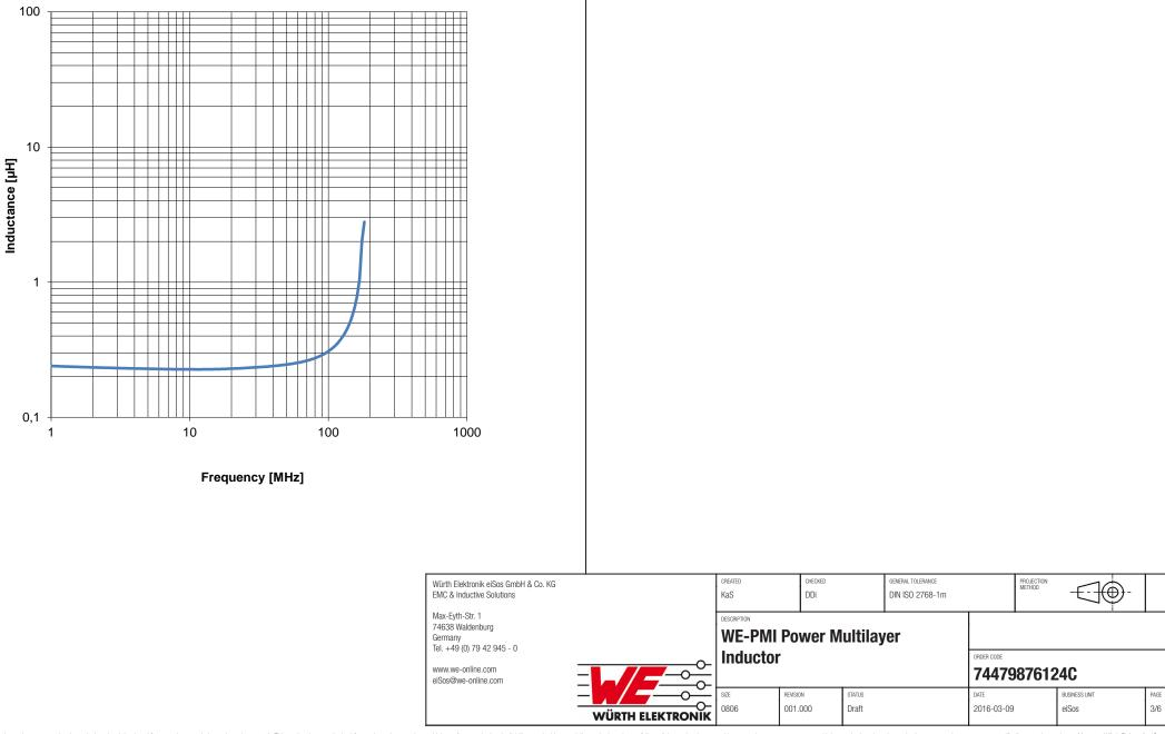
**Typical Inductance vs. Frequency Characteristics:**
