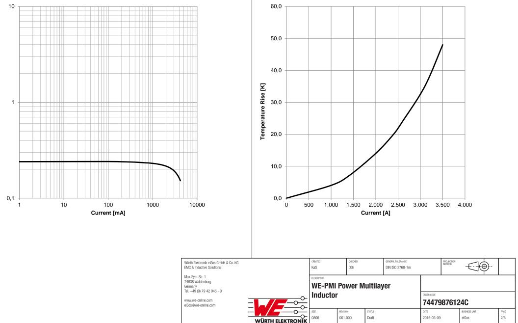
**Typical Temperature Rise vs. Current Characteristics:**
