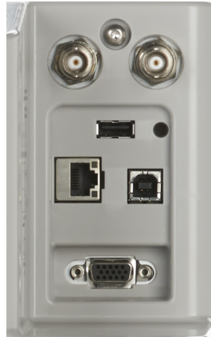
Figure 52. Connectivity section on the back panel.
