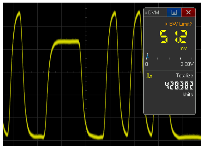
Figure 35. Totalizing the number of runt errors.
