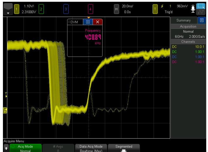
Figure 10. The ultrafast waveform update rate of the 6000 X-Series revealed the existence of rare glitches.
