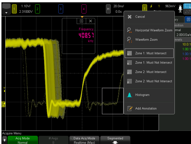
Figure 11. Draw a zone (box) around the anomaly.
