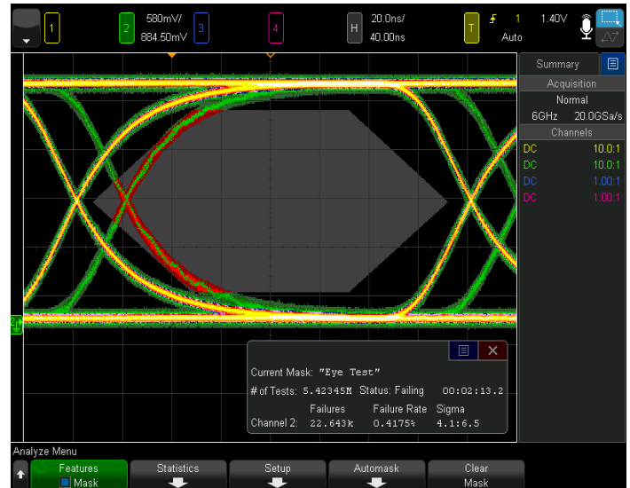
Figure 41. Mask testing of serial data.
