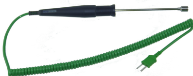
712-8196 - Dual Surface/Immersion Probe - a combined probe for measuring the temperature of running water, radiators and pipes. Temp Range: -50 to 250°C
