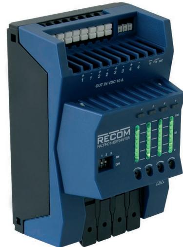
Dimensions (HxWxD): 111.0 x 72.0 x 61.9mm (4.37 x 2.83 x 2.44 inch)
