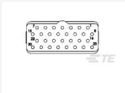
TE Part #1738171-1 INSERT ASY,PIN,E,30-P,KEY B
