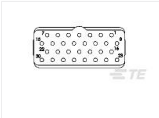
TE Part #1738169-1 INSERT ASY,SOCKET,E,30P,KEY A
