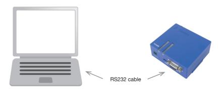
Step 4. Open 'HyperTerminal' on your PC. You will be requested to enter the number of the COM port your are using to communicate between the ZEST and PC. Upon request, ensure the following information is inserted:
