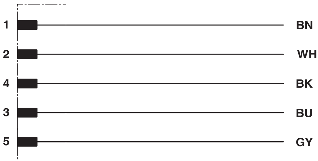
Contact assignment of the M12 plug
